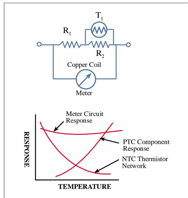
Figure 24: Temperature Compensation
