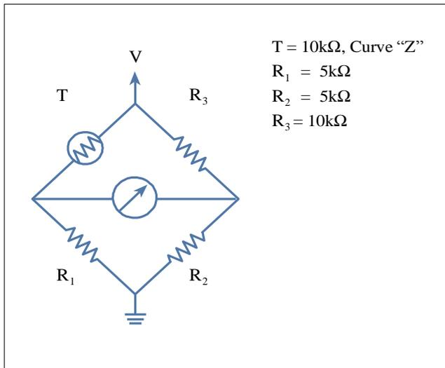
Figure 2: Wheatstone Bridge - Voltage Mode
