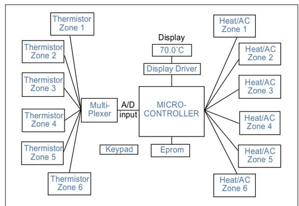
Figure 1: Microcontroller System
