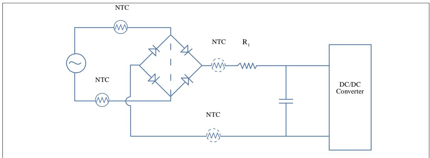
*Figure3 : Surge Current Limiting Circuit For Switch Mode Power Supply.*
