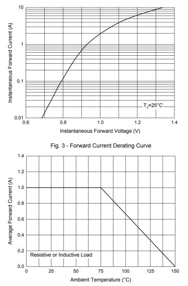
Fig. 1 - Typical Instantaneous Forward Characteristics
