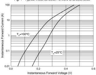
Fig. 1 - Typical Instantaneous Forward Characteristics
