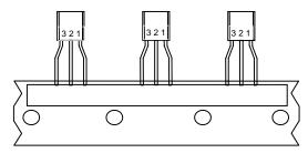
Position of components when being withdrawn
